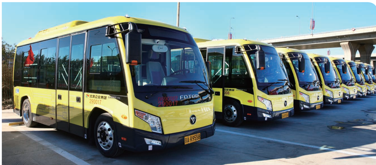
6-meter long pure electric buses used for the operation of micro-circular routes
